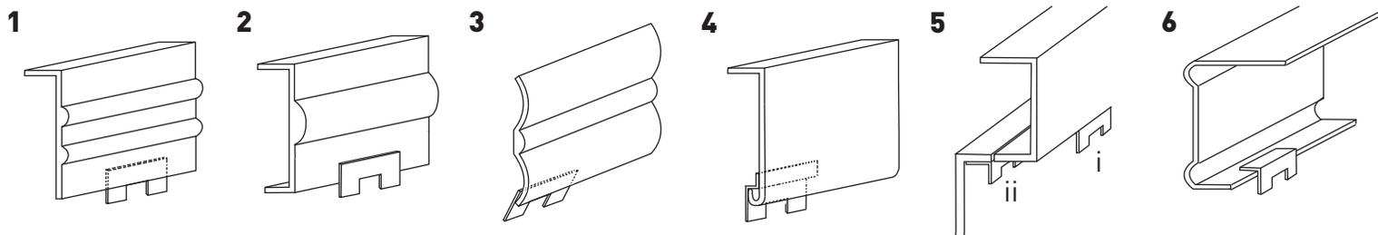
1. "STOP" A - Inside attachment (preferred) - No inner lip on rub rail - Notch in STOP to be mounted flush with rub rail.
