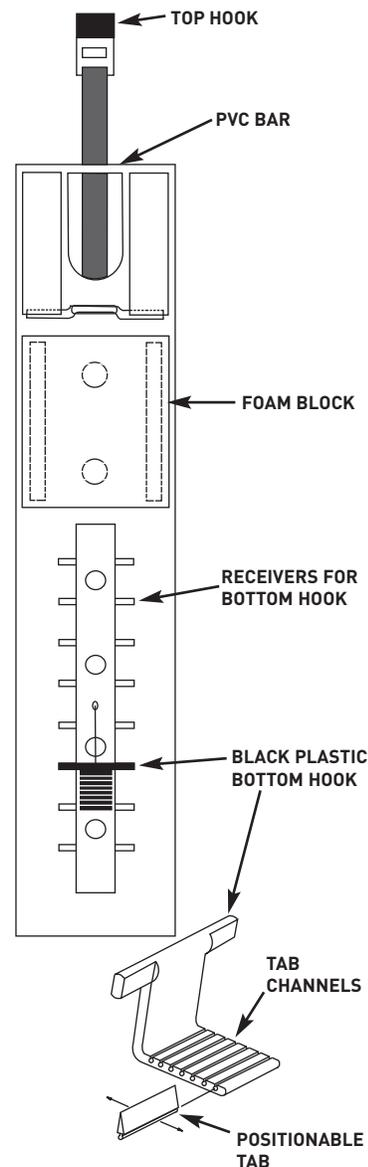
1. "STOPS" A & B notch should be mounted flush with the bottom edge of the rub rail. The legs that stick down from the STOP will prevent horizontal movement of the hook. Your primary strength for attachment should be the plastic hook and tab behind and under your rub rail.
